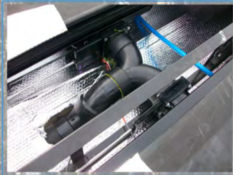
Heated Holding Tanks With Protected Valve System
