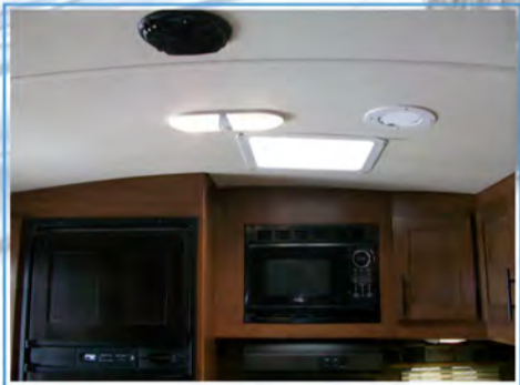
Vaulted Radius Ceiling Providing Approx 5" Addl Headroom
