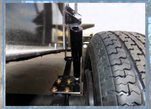
HD Shock Absorbers With XL Shock Plate
