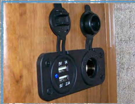
12V Triple Charge Station (Charges iPads and Cell Phones) Plus 12V/USB Ports in Bedroom
