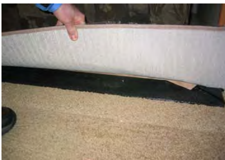
No Insulation Under Slide-Out Carpet
