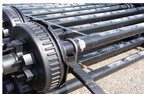
Heavy Duty Axles with Off Road Brake System
