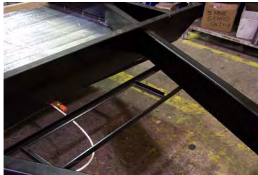
Rugged A Frame (Off Road) Chassis
