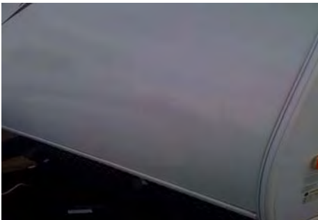
Flat Front Fiberglass Wavy and Soft
