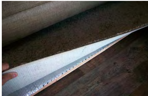
Astro-Foil( R-15) Insulation Under Slide-Out Carpet
