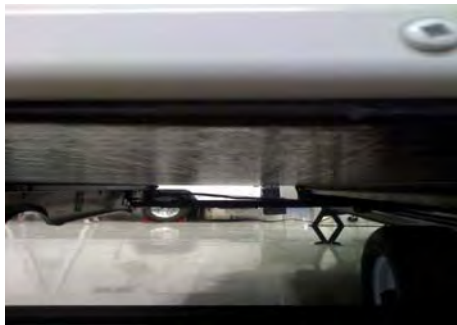
Darco Underneath Slide-Out Tears over Time
